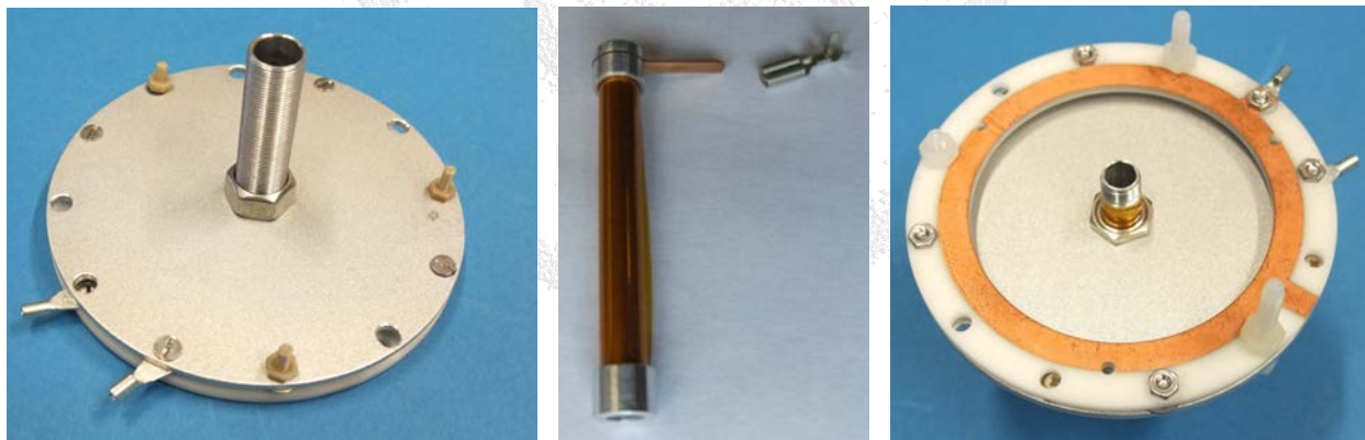
Figure 1.15: Left: rear view of a timing anode with tubing (here DET40/o) for supporting an electrically insulated inner tube (middle picture, with contact lug). After removing the front cap the inner tube can be inserted and shall protrude over the ceramic ring by about 10 mm (right picture). During assembly the detector must be placed on a provisional rear support or on its final mounting gear. Exceptionally, the temporarily placed plastic screws during MCP assembly with ceramic rings may be secured by nuts (MCP stacks with center hole are thicker than the nuts).
