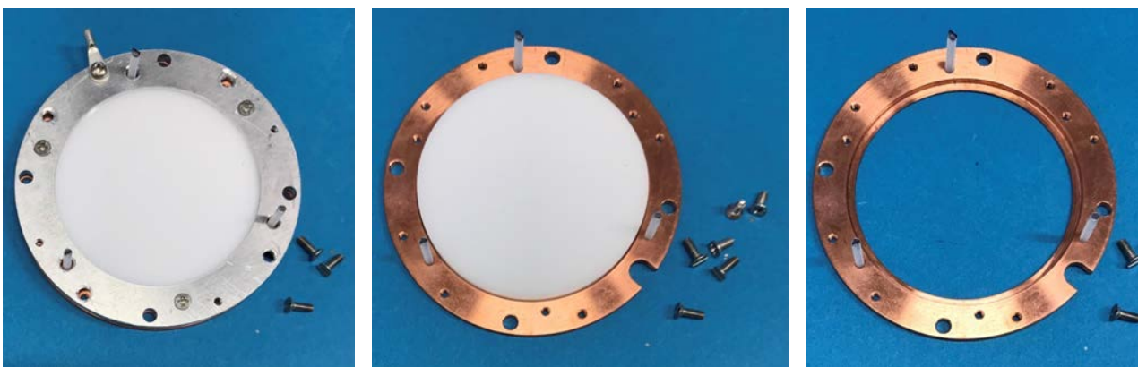
Figure E.1: Pictures of the phosphor screen cage (here: DET40P) at different steps during glass disc (un)mounting. Procedure is similar for DET70(75/80)P DET120P and DET25P (the latter has only 3 screws). For DET40P it is especially important that the 3.2 mm through holes of the cage rings are aligned (if not, rotate the rear ring by 120°).
